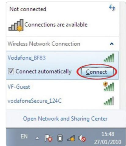
3. When asked for a network security key, type in the **Security Key** also printed on your modem and **Setup Sticker**, then click OK.
